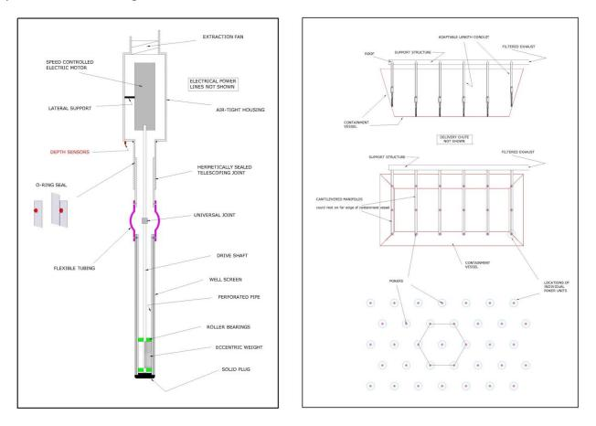
The last sketch suggests how a medium sized vessel such as a railway wagon might be filled with compacted bulk dry particulate cargo in this manner.
